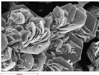
BLH \text{Cs}_{0.2}\text{CoO}_2 \cdot 0.63\text{H}_2\text{O} crystals grown from low temperature molten salt.
